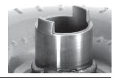
49 Size 13" Daikin Hub Geared Hub Pilot .982" OD x 1.10" L Mounting 6 Threaded Holes Stator Splines 18 Turbine Splines 19
