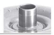
70 Size 11.5" Sachs Hub Smooth Hub W/50 Splines in I.D. Pilot .787" & 1.300" OD Mounting 4 Mounting Nuts Stator Splines 29 Turbine Splines 29
